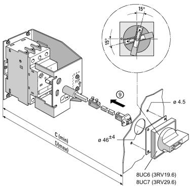
Slide the spacer onto the shaft. Slide the extension shaft into the spacer. Slide the coupling driver onto the extension shaft.
