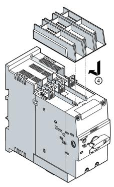
④ Slide the terminal block 3RT2946-4GA07 into the guide tabs provided on the circuit breaker.
