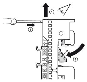
① From the front, insert a screwdriver into the right-hand opening on the busbar adapter and lock the holder (A). The button on the top of the busbar adapter should spring up.
