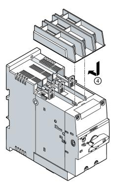
4 Slide the terminal block into the guide tabs provided on the motor starter protector.
