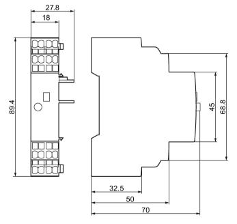
Figure C-42 3RV2921-2M signaling switch (spring-type connection)
