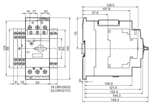
Figure C-12 3RV2.31 motor starter protector (≤ 45 A)
