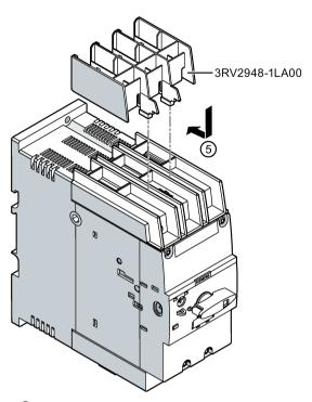
Slide the terminal cover 3RV2948-1LA00 into the openings provided on the terminal block.
