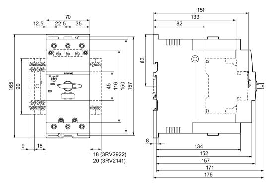
Figure C-15 3RV2.4 motor starter protectors
