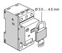
Figure 9-3 Securing the toggle switch (3RV1.1)
