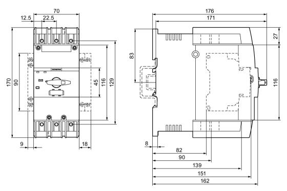
Figure C-16 Circuit breaker acc. to UL 489
