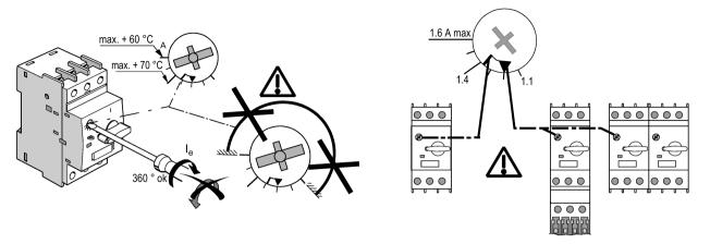
Figure 9-1 Making the current setting I<sub>e</sub>
