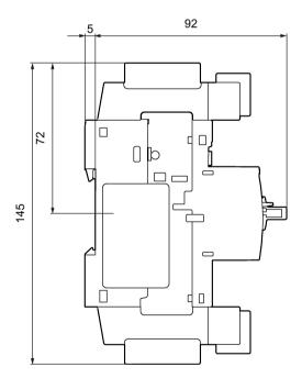
Figure C-10 Circuit breaker acc. to UL 489
