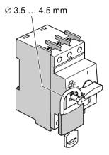
Figure 9-2 Securing the rotary switch (3RV2)
