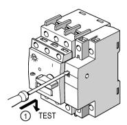
The control circuit must be energized.
