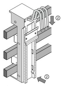
2 Attach the busbar adapter to the busbars from above.
