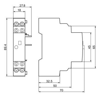
Figure C-41 3RV2921-1M signaling switch (screw-type connection)
