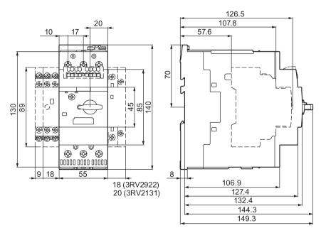
Figure C-13 3RV2.31(≥ 52 A) / 3RV2.32 / 3RV2431-4VA1 motor starter protectors.
