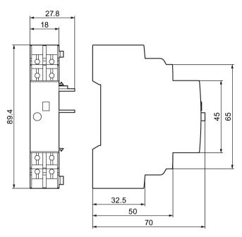
Figure C-43 3RV2921-4M signaling switch (ring cable lug connection)
