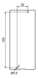
Figure C-17 3RV2.4 motor starter protectors
