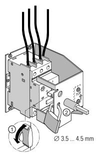
The mechanism can be locked inside the control cabinet with a padlock. The motor starter protector must be set to the O position first, before the lock is attached.
