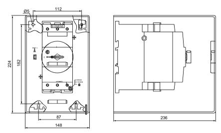
Figure C-44 3RV1946-3A remote motorized operating mechanism
