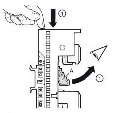
① Press the button on the top of the busbar adapter to release the holder. The holder (A) should flip out from the front of the busbar adapter.
