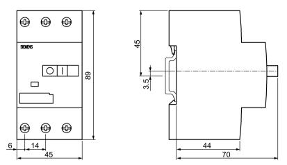
Figure C-3 3RV1611-0BD10 circuit breaker for fuse monitoring, screw-type connection technology S00
