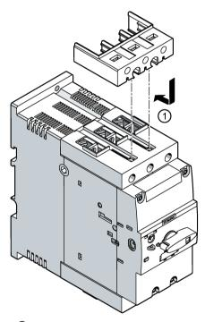
① Slide the terminal cover for the box terminal block into the openings provided on the box terminal block of the motor starter protector.
