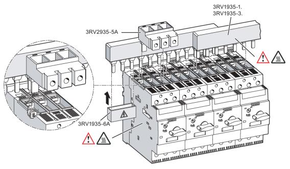
Figure 10-9 Mounting with 3-phase busbar (size S2)
