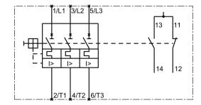
Circuit breakers for fuse monitoring / voltage transformer circuit breakers for distance protection
