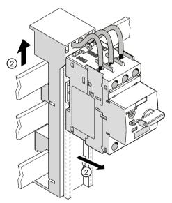
② Remove the busbar adapter from the busbars. To do this, you will first need to push it up slightly so that you can remove it by pulling it off toward you.
