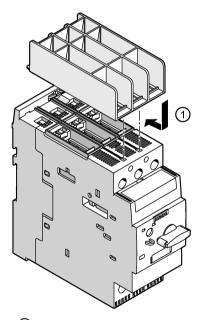
① Slide the phase barriers into the guide rails provided on the motor starter protector.
