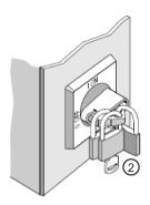
10.8 Door-coupling rotary operating mechanism (not for 3RV1)
