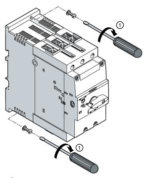
① Using two M4 screws (maximum tightening torque 1.2 to 1.4 Nm) and plain washers, diagonally screw the motor starter protector tight into the designated drill holes.
