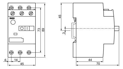
Figure C-4 3RV1611-1.G14 voltage transformer circuit breakers for distance protection with screwtype connection technology, S00
