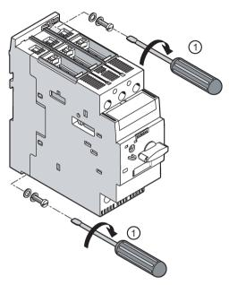
① Using two M4 screws (maximum tightening torque 1.2 to 1.4 Nm), plain washers, and spring washers, diagonally screw the motor starter protector tight into the designated drill holes.
